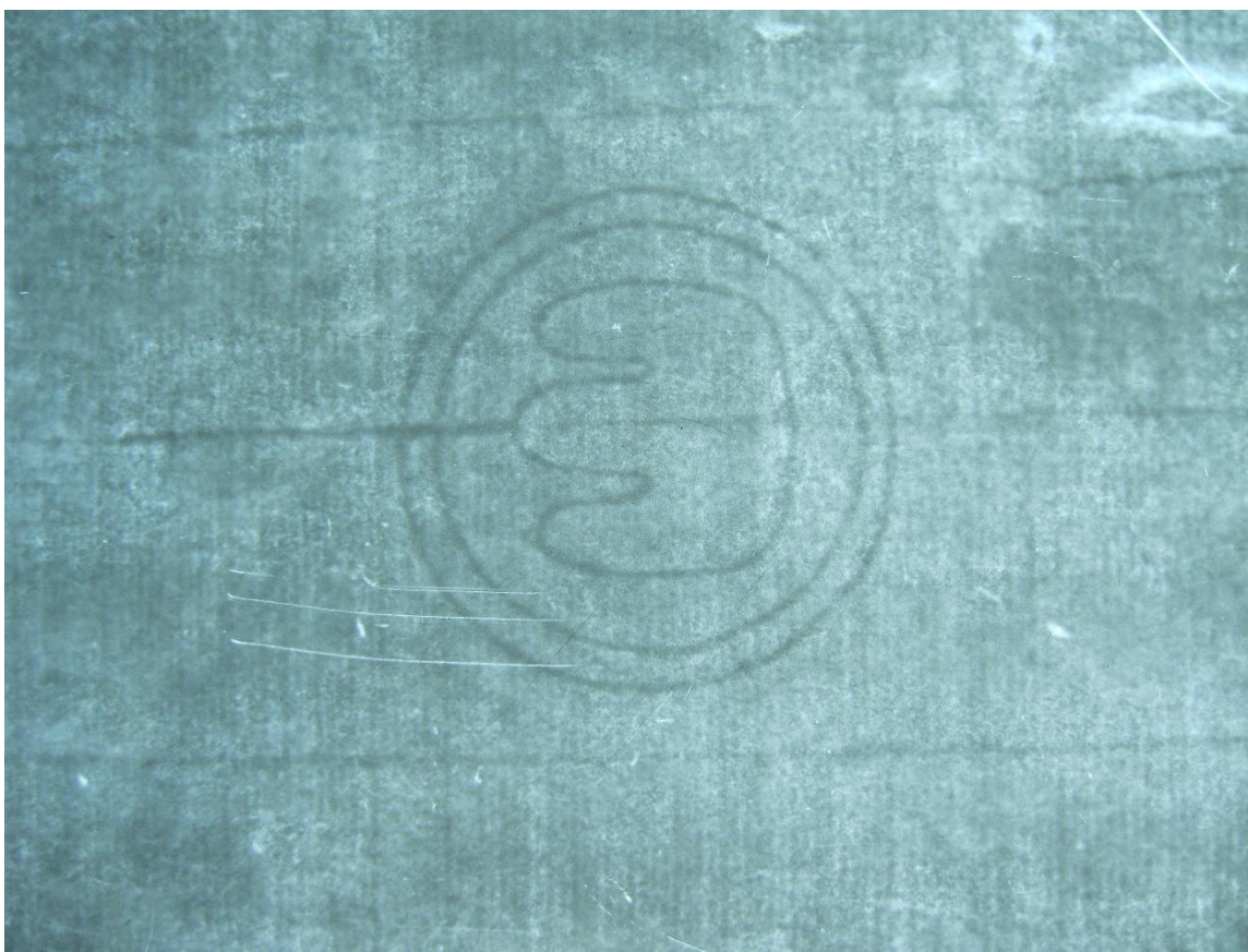
Fig. 2 Beta-radiography of the watermark under investigation
